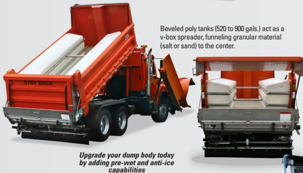
Beveled poly tanks (520 to 900 gals.) act as a v-box spreader, funneling granular material (salt or sand) to the center.
