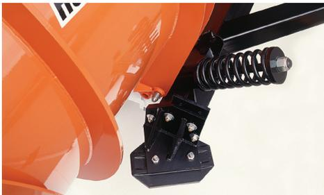
Two adjustable shoes assure proper push frame support. Wear shoe is bolt-on for easy replacement. Two slotted trip springs adjust easily for changing conditions. Two position adjustments for proper attack angle, 45° for standard cutting edge or 30° for carbide cutting edge.
