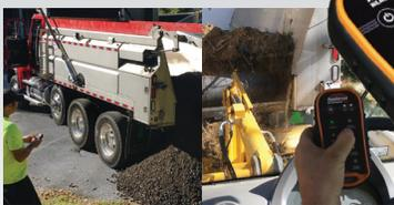
The B-Maxx™ Command Remote over-rides the standard controller to allow the operator greater freedom of movement...or operation from other equipment such as a skid steer loader.
