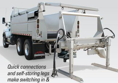
Quick connections and self-storing legs make switching in & out of winter-duty simple.
